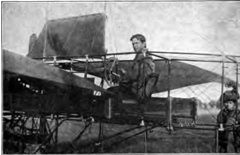
Fig. 53. Fairchild Monoplane with Frame of Steel-Tube Construction
